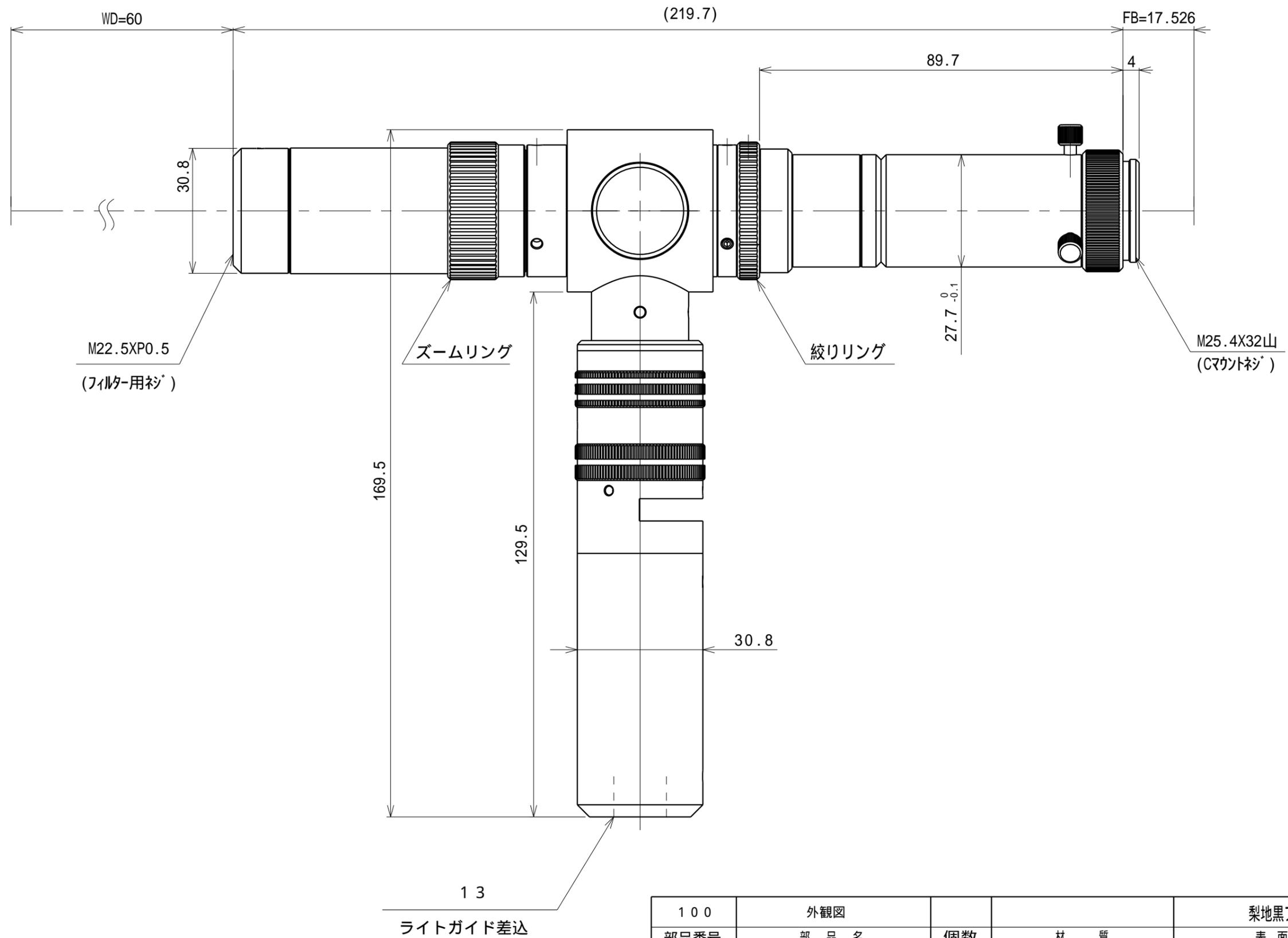
KCM-Z6D : 倍率 = 1.0 ~ 6.0倍 W.D. = 60mm
